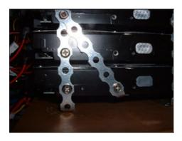
Note nice usage of construction metal stripes with holes which is usually used to hold fence. It has holes just the right size for screws to go through and hold disks nicely spaced (although a little bit more space would be ideal). It's soft enough to be bent at corners to produce nice and leveled space between it and case.
