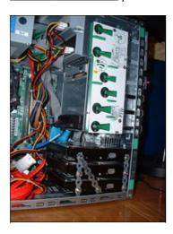
Final position in case, notice empty space above 4th disk which was occupied by disks before (which didn't have enough airflow because of that)
