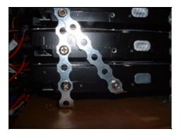
Note nice usage of construction metal stripes with holes which is usually used to hold fence. It has holes just the right size for screws to go through and hold disks nicely spaced (although a little bit more space would be ideal). It's soft enough to be bent at corners to produce nice and leveled space between it and case.
