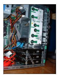
Final position in case, notice empty space above 4th disk which was occupied by disks before (which didn't have enough airflow because of that)
