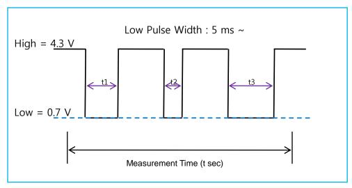
Fig.5 Dust sensor Low Ratio
