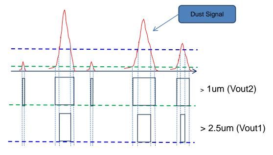
Fig.3 Detection Size Determination
