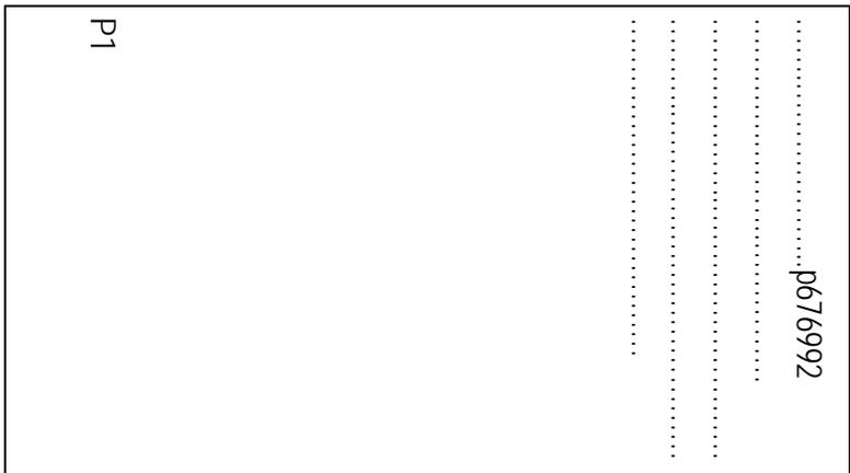
This is a representation of the downloading of 648x1016 points = 676992 pixels (p1 being the first transmitted pixel).
